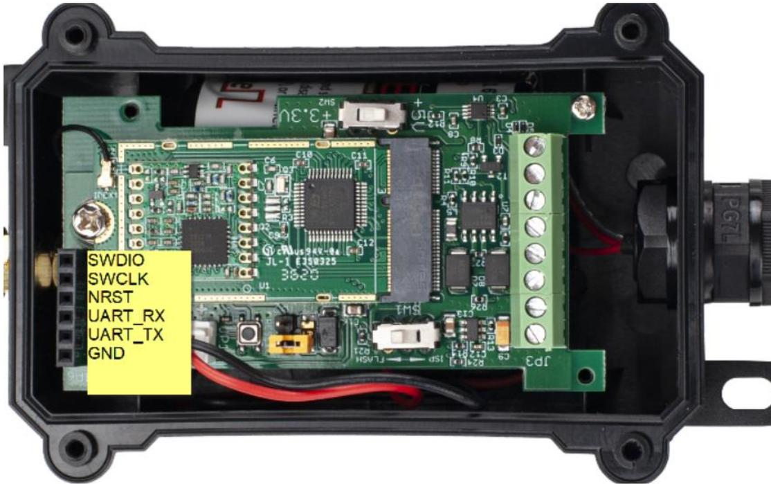
In the PC, you need to set the serial baud rate to **9600** to access the serial console for LDDS75. LDDS75 will output system info once power on as below:
