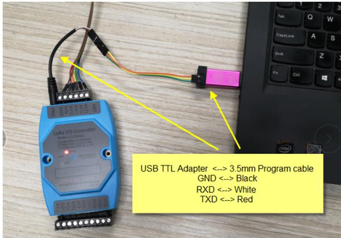
In the PC, you need to set the **serial tool** (such as [putty](#), SecureCRT) baud rate to **9600** to access to access serial console for LT.
