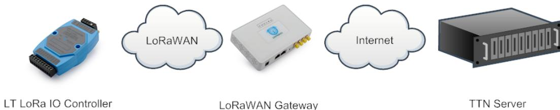
The LG308 is set up by default to connect to the [TTN network](#), so it is simply necessary to configure TTN Server to recognise the device.
