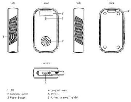
**Note:** the environment and orientation of the device can influence the radio performance. For optimum results keep the zone around the antenna area clear from any conducting material or magnetic fields.
