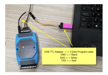
In the PC, you need to set the **serial tool** (such as <u>putty</u>, SecureCRT) baud rate to **9600** to access to access serial console for LT.
