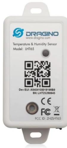
The Dragino LHT65 Temperature & Humidity sensor is a Long Range LoRaWAN Sensor. It includes a **built-in SHT20 Temperature & Humidity sensor** and has an external sensor connector to connect to external sensors such as **Temperature Sensor, Illumination sensor, Interrupt Sensor, ADC sensor etc** .
